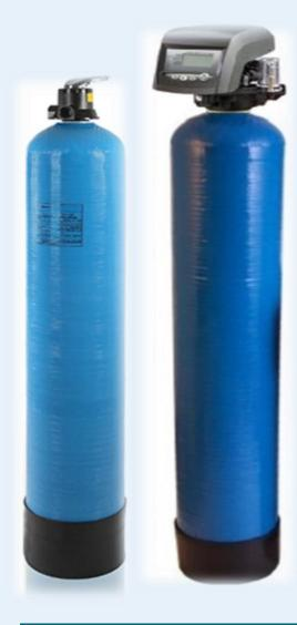
Yasric - Sand Filters are commonly used in most standard residential and commercial water filtration systems for removal of suspended solids and turbidity. Water 2000 Inc. provides both In-Depth filter and Multimedia Filters. In-Depth filters remove debris down to 20-30 micron while Multimedia filter removes debris further down to 10 micron.
